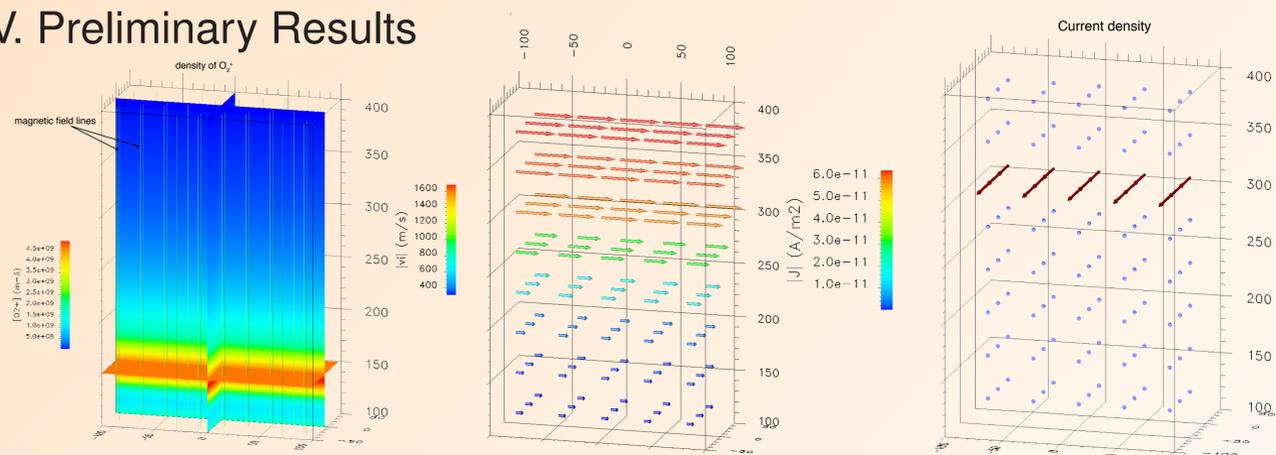
Figure 4: Example of diagnostics for  $\vec{U}_n=0, B_z=20$  nT.
