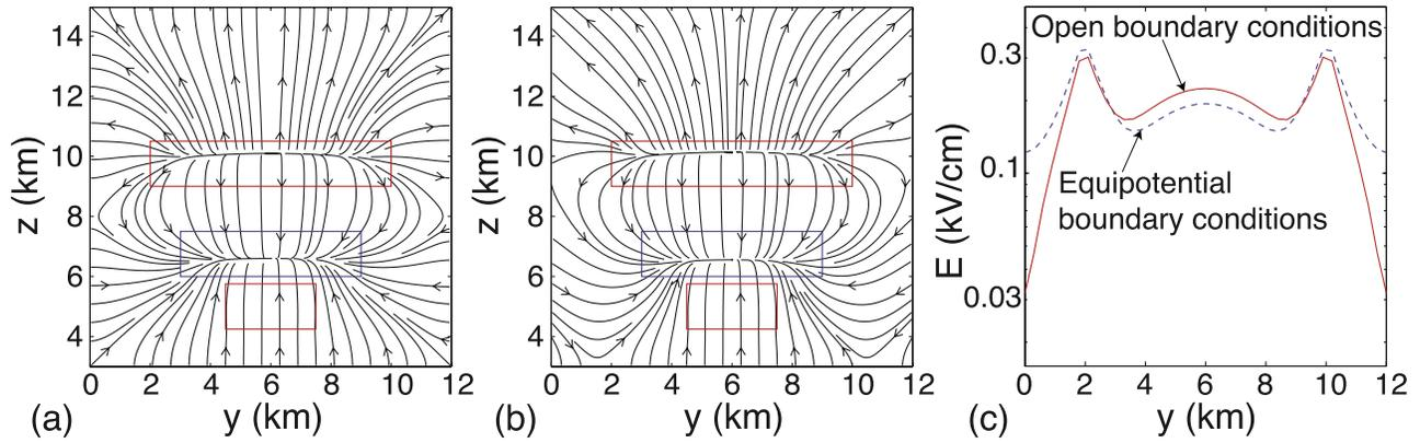
**Figure 3.** Electric field lines pattern of the thundercloud with parameters specified in Table 1 in a simulation domain with (a) equipotential boundaries and (b) open boundaries. (c) Comparison of the electric field magnitudes using equipotential (dashed line) and open boundary conditions (solid line) at an altitude of 9.8 km.
