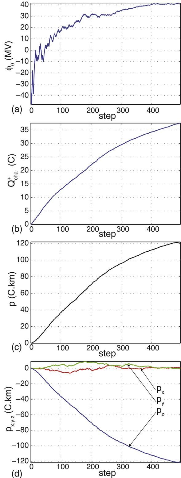
**Figure 9.** Parameters of the simulated discharge shown in Figure 4 at each step of the development: (a) channel potential  $\phi_0$ ; (b) charge carried by the positive leaders  $Q_{chna}^+$ ; (c) magnitude of the discharge electric dipole moment  $p = |\vec{p}|$ ; and (d)  $x$ -,  $y$ - and  $z$ -components of the dipole moment  $\vec{p}$ .
