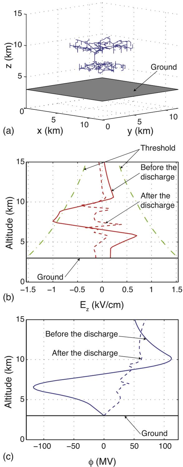
**Figure 8.** (a) Three-dimensional view of the intracloud discharge shown in Figure 4 after 496 steps. (b) Electric field before the flash (solid line) and after (dashed line) along the central vertical axis of the simulation domain. The electric field initiation threshold is shown for reference by dash-dotted lines. (c) Electric potential before (solid line) and after (dashed line) the discharge development along the same axis.
